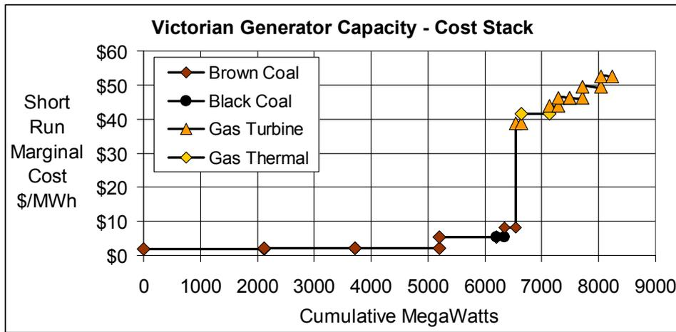
Up to 6,000MW of Victorian energy may be dispatched from cheap brown coal, but rapid changes or increases in demand cause a dramatic rise in costs as gas is called into action.
