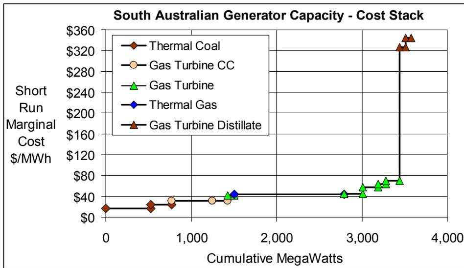
In South Australia, only 500MW comes from cheap coal and variations up to 1,000MW in wind power need gas turbines to follow the variations. Above 3,500MW of demand, the costs rise -- becoming 6 times as expensive as the most expensive Victorian electricity.
