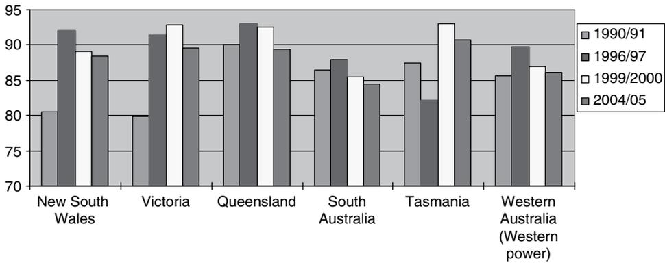
Fig. 11.7. Power stations' availability to run. Source: ESAA, Electricity Gas Australia 2006.
