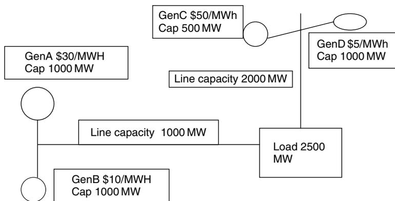
Fig. 11.12. Illustration of Four Generators and Two Transmission Lines Serving a Load.
